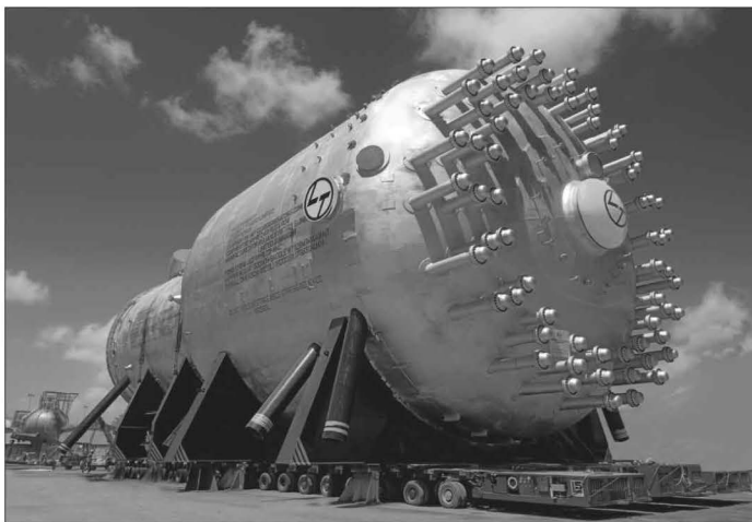
The world's largest FCC regenerator built at L&T's Hazira Works
